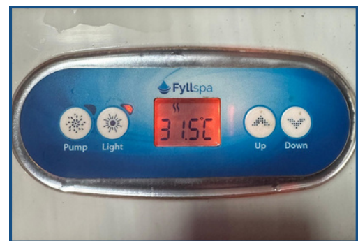
Hot Tub Control Panel
